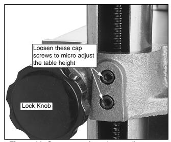
Figure 12. Cap screws for column adjustment.
